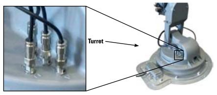
4 Remove the bolt holding the cable harness to the unit, and detach the cable harness from the lift arm.
