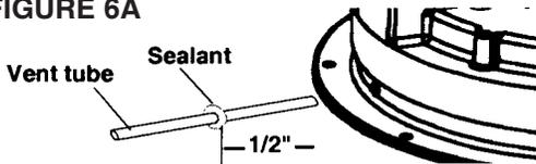
**CAUTION: DO NOT GET** sealing compound between Base Plate and Rotating Gear Housing. **DO NOT PAINT** top of Base Plate or around Rotating Gear Housing.
