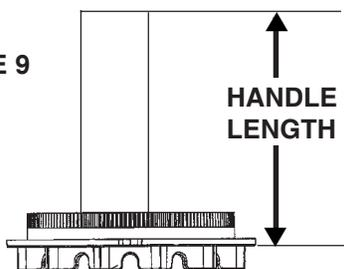
**STEP 15.** The directional handle and threaded rod will fit roofs up to 5-1/4" thick. If you are using wedges to compensate for roof/ceiling slope, be sure to allow for this extra thickness. You may add an extension to the directional handle for thicker roofs. Each extension will increase the length of the directional handle by 2-1/4". Figure 11
