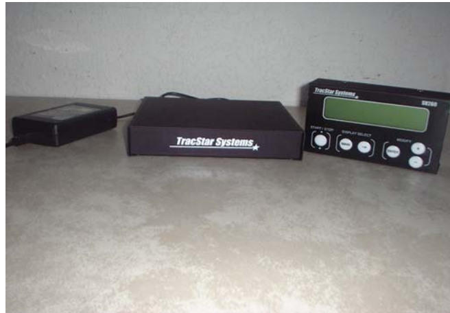
Figure 1.4-2 SV360 Power Supply, Indoor Box and Display Unit
