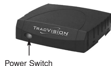
Receiver Front Panel Power Switch
